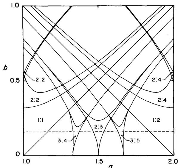
Fig. 2. Locally stable phase locking regions for (1). The dashed line at  $b = 1/2\pi$  separates the regions in which (1) is a monotonic function of the unit circle ( $b < 1/2\pi$ ) and a non-monotonic function ( $b > 1/2\pi$ ). In the non-labelled regions are phase locked, quasiperiodic and chaotic dynamics (see text).
