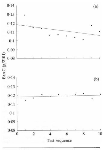
FIGURE 1 Regression line showing the variation of breath alcohol concentration with test sequence. (a) Subject 1 (SEE = 0.0076, BrAC = -0.00141T + 0.118); (b) Subject 9 (SEE = 0.0025, BrAC = 0.00039T + 0.117).
